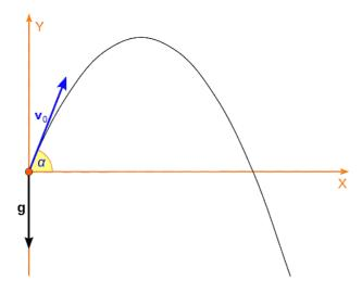
Given the launch angle  $\alpha$  (radians) and the initial velocity  $v_0$  (ms<sup>-1</sup>), the projectile follows a parabolic trajectory represented by the following equation:
